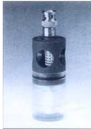
Detector cell with electrolyte reservoir and connection for BNC plug. 20 ml electrolyte supply sufficient for 12 months continuous operation.
