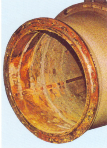
Carbon steel centrifuge bowl after 1 year of operation.
