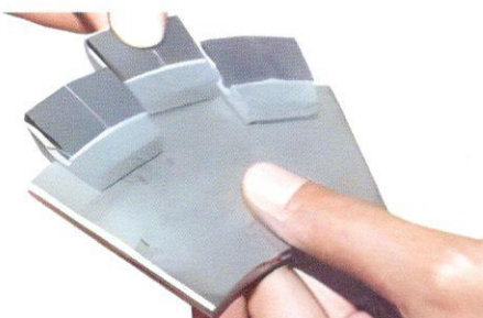
Super-D-Canter scroll showing the tungsten carbide tiles in position.
